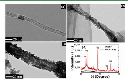
Figure 2. (a) TEM images of one single CNT from the VACNT hexagonal network. One single CNT electrodeposited with CdS QDs after (b) 2 min and (c) 5 min, respectively. (d) XRD spectra of pure VACNT and after 5 min of electrodepositing with CdS QDs.
