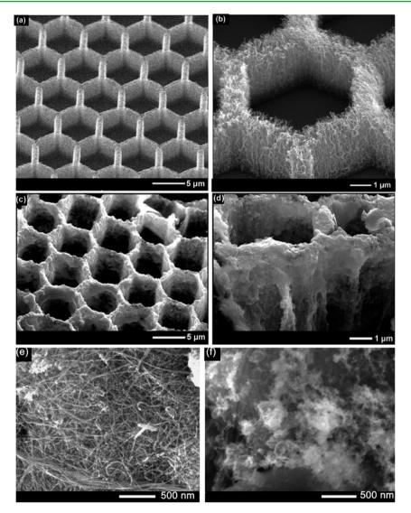
Figure 1. (a) Low and (b) high magnification SEM images of the VACNT hexagonal network. (c) Low and (d) high magnification SEM images of the VACNT hexagonal network after 5 min of electrodepositing with CdS QDs. (e) SEM image of the screen-printed CNTs. (f) SEM image of the screen-printed CNTs after 5 min of electrodepositing with CdS QDs.
